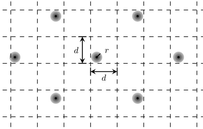
Fig. 2: A visualization of the space subdivision. Each radially shaded disk has width  $r$ , the upper bound of the error  $\|\mathbf{e}\|$ . Each cell has width  $d$ , chosen to be between  $\|\mathbf{e}\|$  and  $\lambda_1(L)/\sqrt{m}$ . Note that the grid intersects the left-most disk, potentially leading to an error in the reduction.
